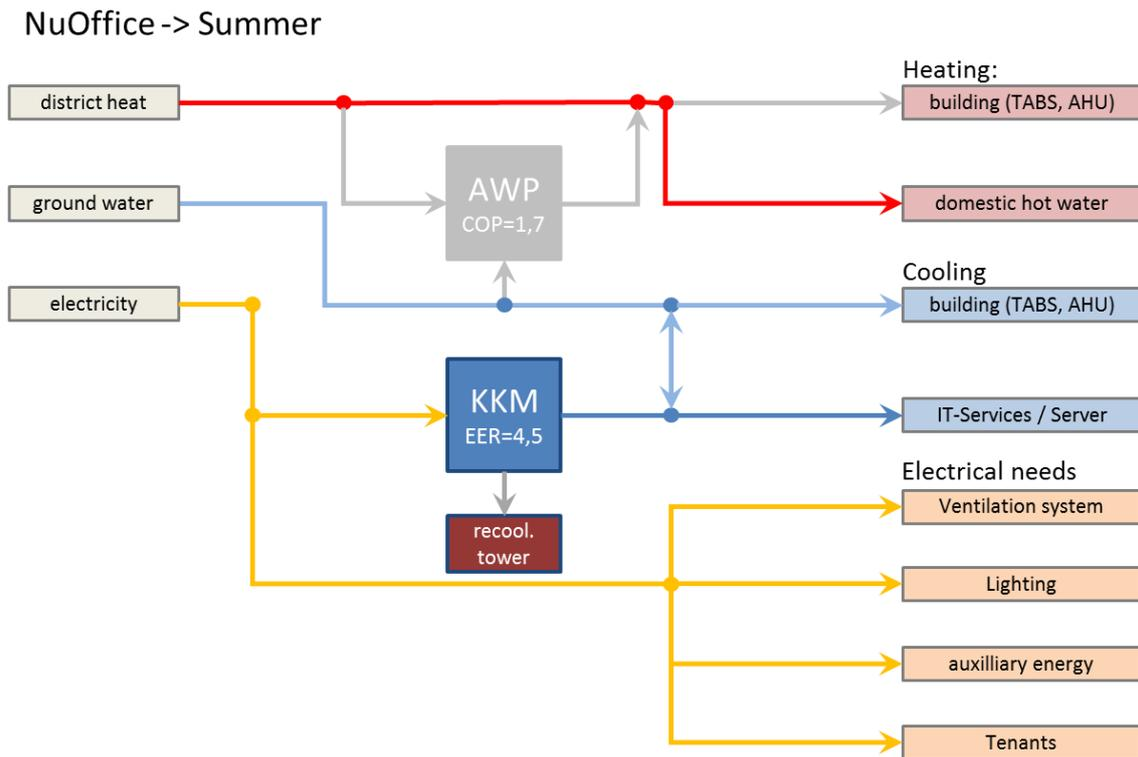
Figure 2: Overview of the installed technical devices and their energy fluxes in case of summer.
