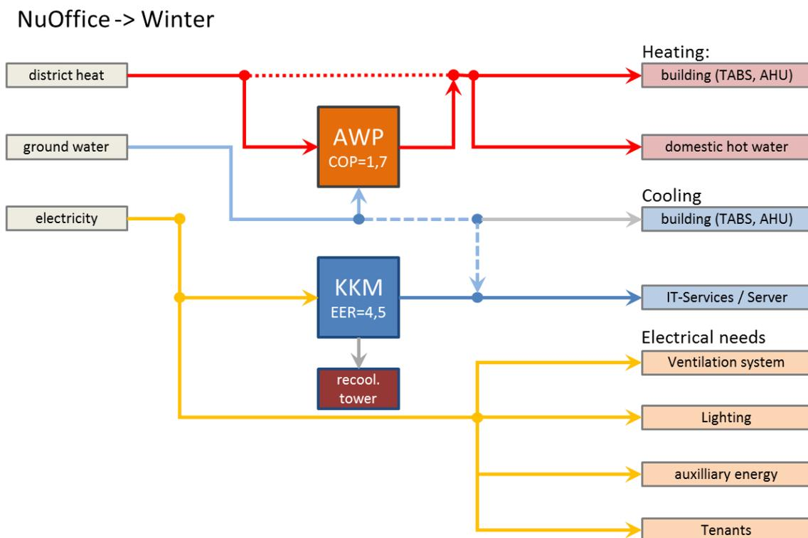
Figure 1: Overview of the installed technical devices and their energy fluxes in wintertime.
