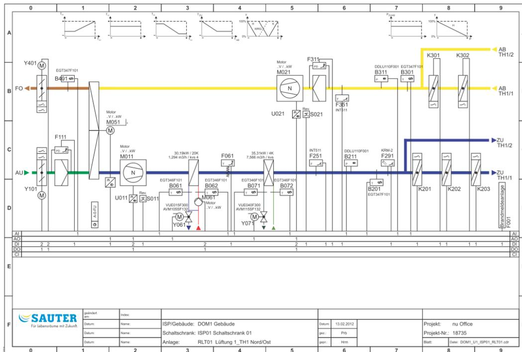
Figure 6: Scheme for one AHU as visualized in the control unit.
