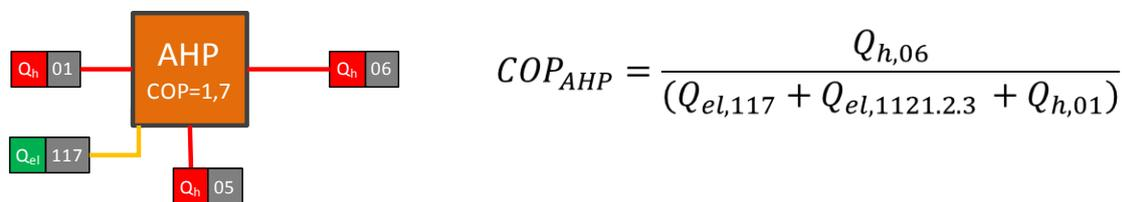
Figure 9, Performance of the Absorption Heat Pump.
