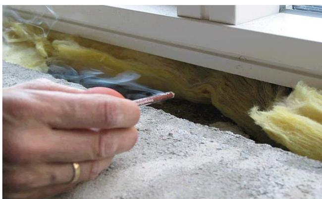
Fig. 2.3.2: Example of registration of white smoke movement to trace cracks and crevices in combination with the blower door test.
