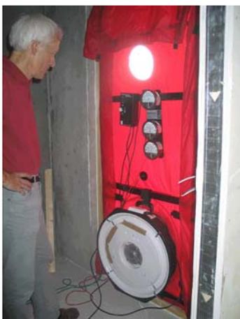
Fig. 2.3.1: Blower Door test in an apartment.
