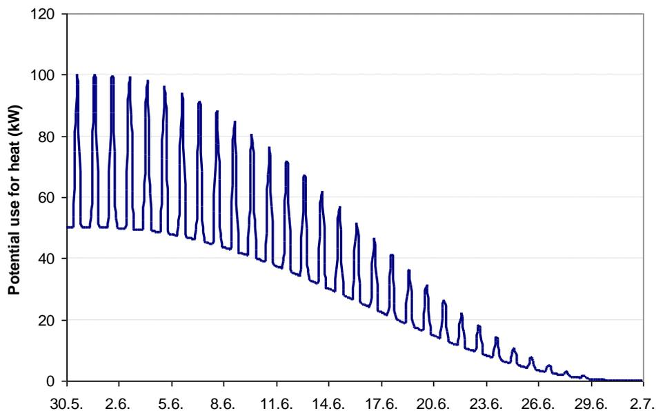
Figure 13. Potential of the greenhouse to use extra heat.
