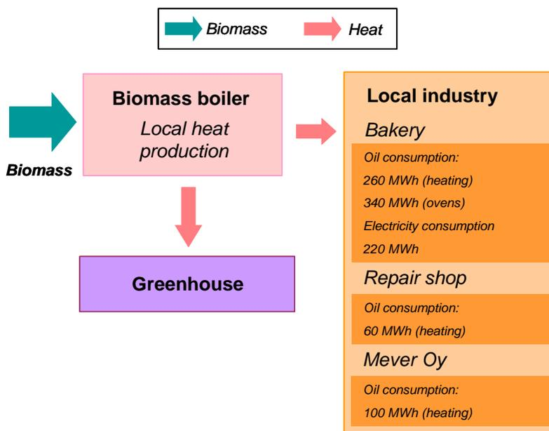
Figure 9. Energy system in the case of biomass boiler producing heat to industrial demand.
