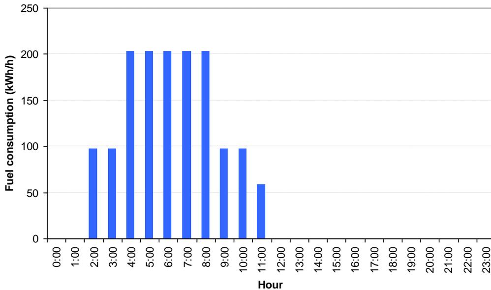
Figure 12. Fuel consumption of the bun ovens in the bakery.
