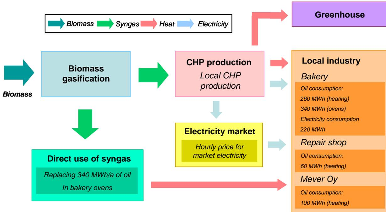
Figure 8. Description of the Härsilä energy system with gasification plant and CHP engine.
