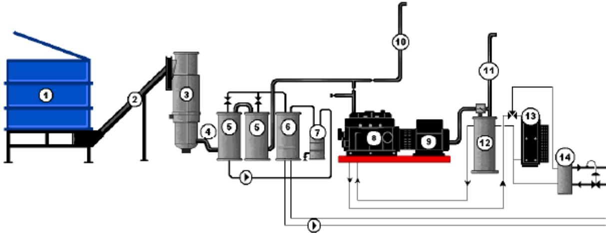
Figure 5. Scheme of Gasification CHP: 1) fuel storage, 3) pyrolyse reactor, 5) syngas washer 6) wash water tank, 8-9) gasengine + generator, 12-13) heat recovery.
